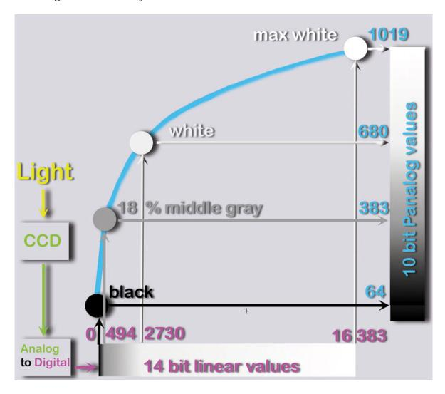
The Panalog curve converts 14 bit linear to 10 bit log
